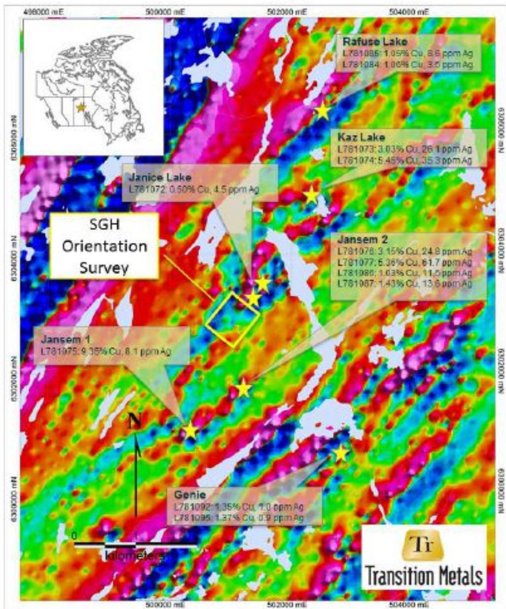
Figure 1: Location of selected grab samples reported in Table 1 and known copper occurrences overlain on an image of a horizontal derivative of total field magnetic intensity, re-processed from 1992 airborne geophysical data.
