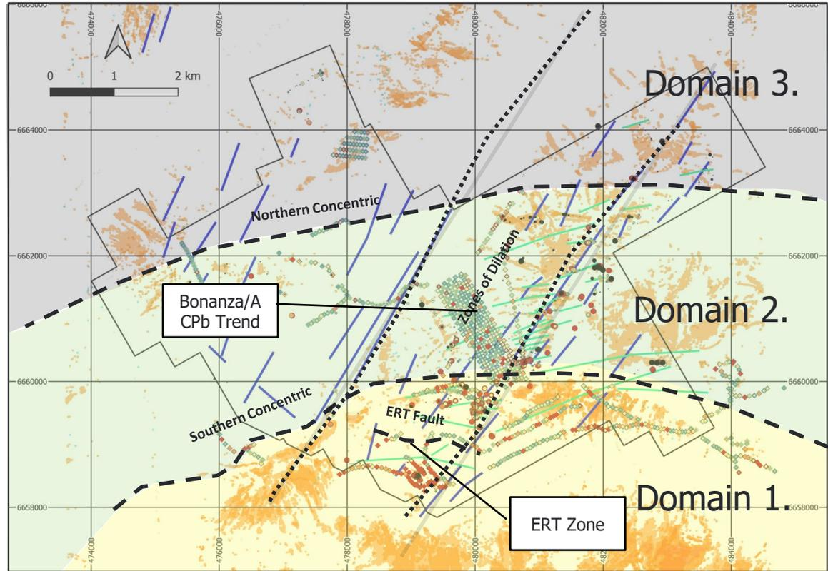
Elevated Au-Ag in rocks, soils, argillic alteration and lineaments
