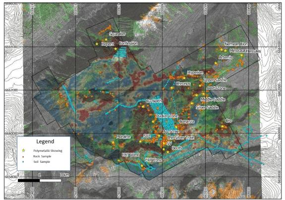
XTM:TSXV \*ASIG Mag and Propylitic (Green), Sericitic (Orange), and Py/Hem (Red) multispectral alteration polygons
